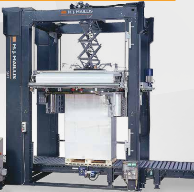
Tilting roll support for very easy film loading
