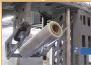
Tilting roll support for very easy film loading
